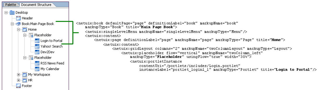
Figure 3 Hierarchical structure of a portal desktop
